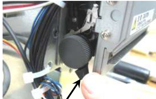
Head Up Lever shown in the “down” or closed position. Pertains to the MTP-2822, the MTP-2832, and the MTP-2242
